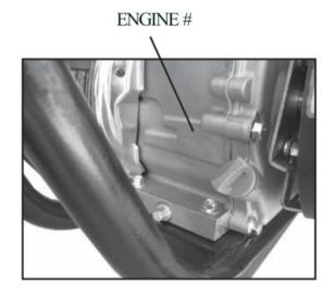
The engine number is located on the bottom front portion of he Mini Bike Engine.
