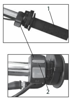
Right Throttle Grip(1): The engine speed is regulated by the position of the right throttle grip. Throttle is increased by turning the throttle grip toward the operator. Engine speed is decreased by turning the throttle grip away from the operator.
