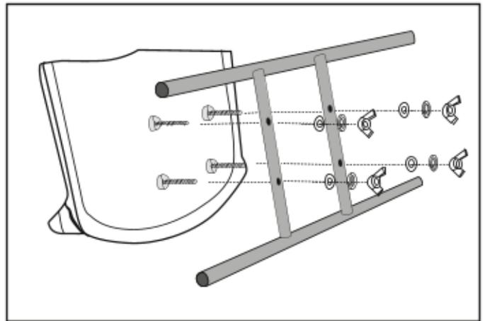
**7. Attach the seat frame to the pontoon frames.**
