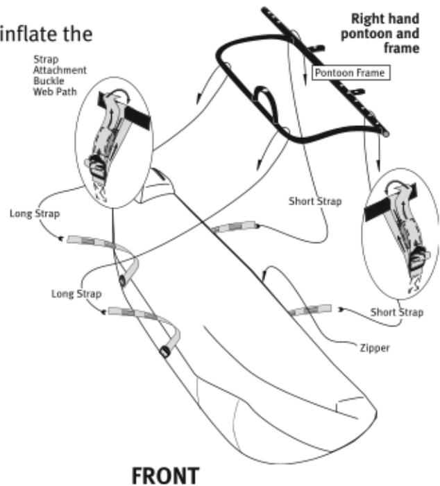
Now attach the two inside and two outside webbing straps on the pontoon to the pontoon frame. Thread the straps as follows:
