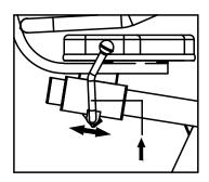
Raise the lever and then slide forward or backward to adjust the seat.
