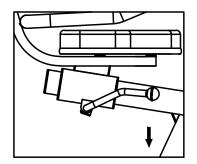
After getting the right seat position, push the lever down to lock the seat in place.
