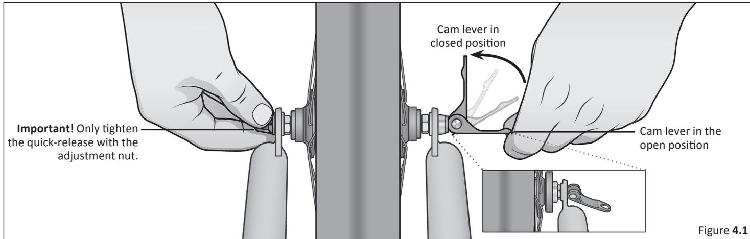
1. A hollow axle with a shaft **skewer** running through it which has an adjustable tension nut on one end and an over-center cam on the other (cam action system, **Figure 4.1**)
