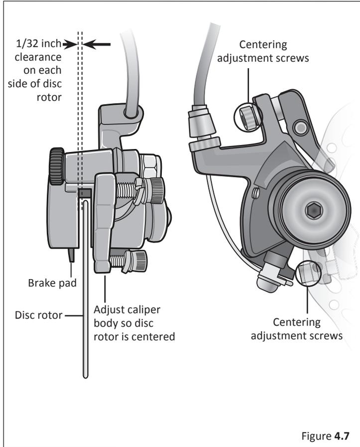
Example of Brake Cable Connected to Brake Arm
