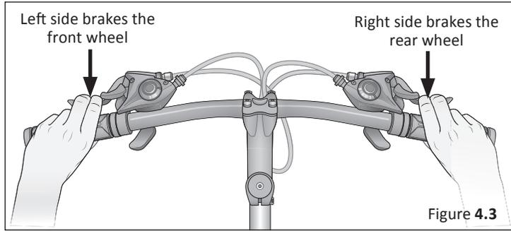
to check how your bike's brakes are set up, squeeze one brake lever and look to see which brake, front or rear, engages. Now do the same with the other brake lever.
