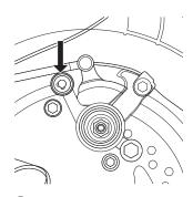
**3** If the disc brake is dragging on the brake pads, use your fingers to twist the caliper adjuster in either direction until disc is centered between the brake pads.
