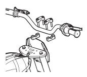
**1** Place the handlebars in the handlebar clamps.
