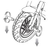
**1** Loosen axle bolt using a 14 mm and a 17 mm socket wrench. Slide axle bolt out and remove front wheel.
