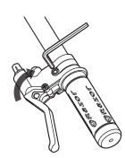
**3** Adjust the brake levers to the proper place and tighten it with the 5 mm Allen wrench.
