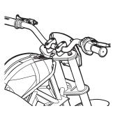
**2** Align with the front fork and tighten the bolts using a 6 mm Allen wrench. When properly tightened, the handlebars should not move forward or backward.
