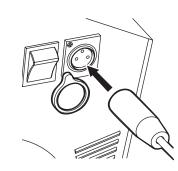
**2** Plug the charger into the charger port. The light on the charger should turn red during charging then back to green when charging is complete.
