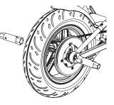
**2** Using a 17 mm and 14 mm socket wrench, loosen the nut and axle bolt on the front wheel.
