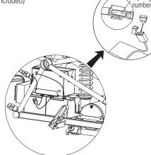
**2** Locate the fuse box attached to the batteries. Check fuse to see if the fuse is burned out. Remove damaged or burned fuse and replace with a new one of equal amperage.
