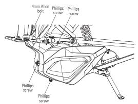
**1** Loosen the 4mm Allen bolt and the four (4) Phillips screws on the battery cover. Remove cover.
