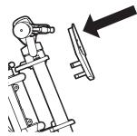
**1** Align the two (2) tabs on the plate with the holes on the front fork and carefully push inward until plate clicks securely into place.
