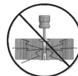
This icon warns you to not over tighten your bolts. This is to prevent structural damage and also splintering your wood.
