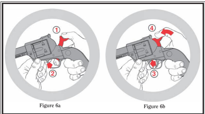
The revolver is now in its normal carrying condition -- hammer and trigger fully forward and transfer bar lowered out of the firing position.
