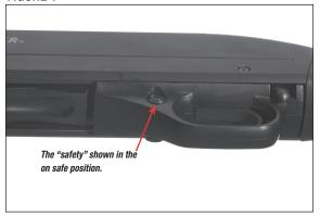
The cross bolt "safety" is designed to prevent the trigger from being pulled when in the on safe position. The "safety" is located at the front of the trigger guard. In the off safe position, a red warning band is visible on the "safety" button on the left side of the trigger guard. It is essential that you become very familiar with the feel, look and operation of the "safety" on this shotgun before attempting to load and shoot.
