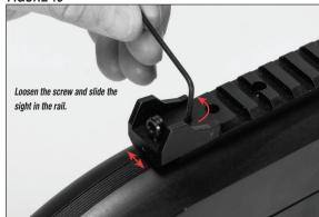
4. Tighten the Allen screw on the right side of the sight. Do not overtighten.
