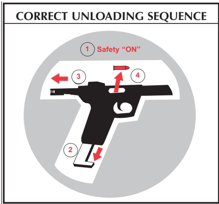
4. The gun is now unloaded. If it is desired to close the bolt on an empty chamber, visually inspect to ensure the chamber is empty. Ensure that the magazine is not in the pistol and that the safety is "on," retract the bolt to its rearmost position, release it, and the bolt will snap forward. Keep your fingers out of the receiver!
