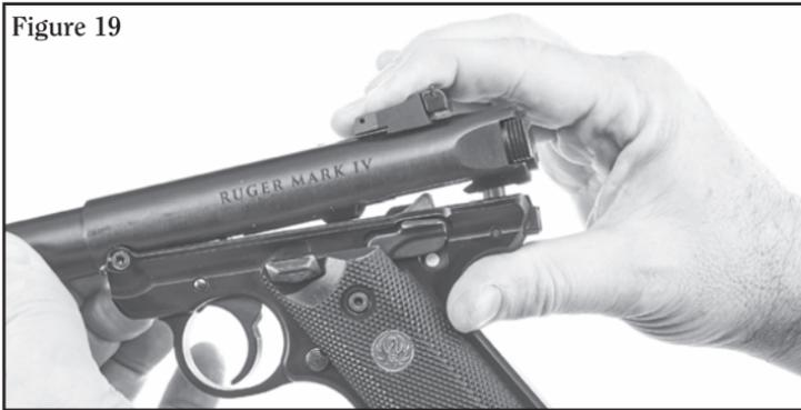
6. Replace the empty magazine into the magazine well, **point the pistol in a safe direction**, place the safety in the “off” position to expose the red dot, and pull the trigger to uncock the gun. **Guns should not be stored loaded or cocked.**
