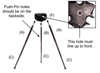
STEP 6: Slide Part (D) (3X) through the holes in the Tri-Pod Base (F) slot holes and tighten nut (E) (3X).
