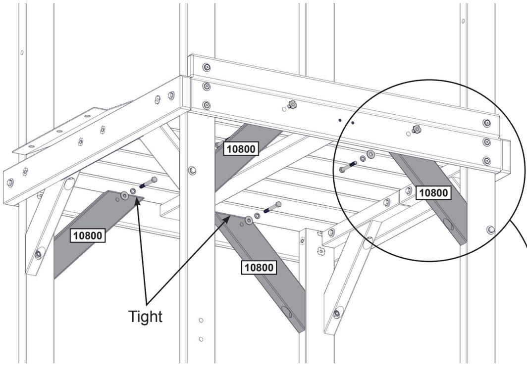
**Assemble T-Nuts first with hammer!**
