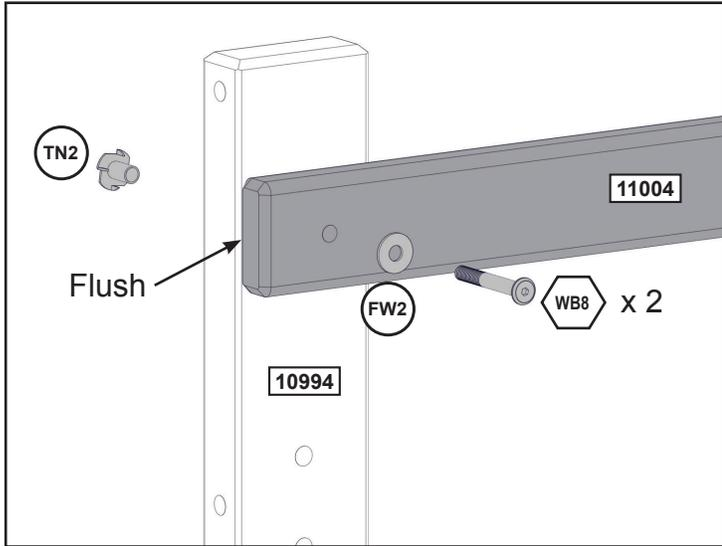
Assemble T-Nuts first with hammer!
