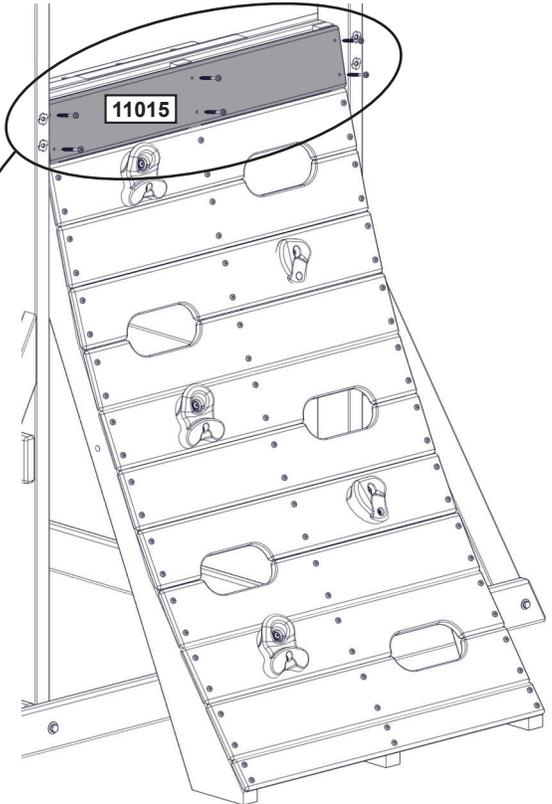
Pre-drill S7 holes using a 1/8" drill bit.
