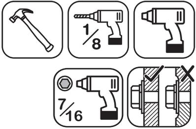
**Assemble T-Nuts first with hammer!**
