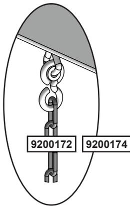
**Caution:** Threaded Quick Links must be installed with the gate completely down covering the threads and tighten as instructed.
