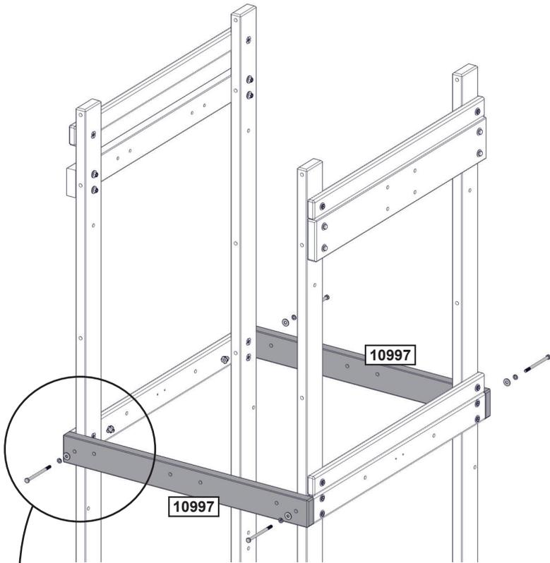
Assemble T-Nuts first with hammer!
