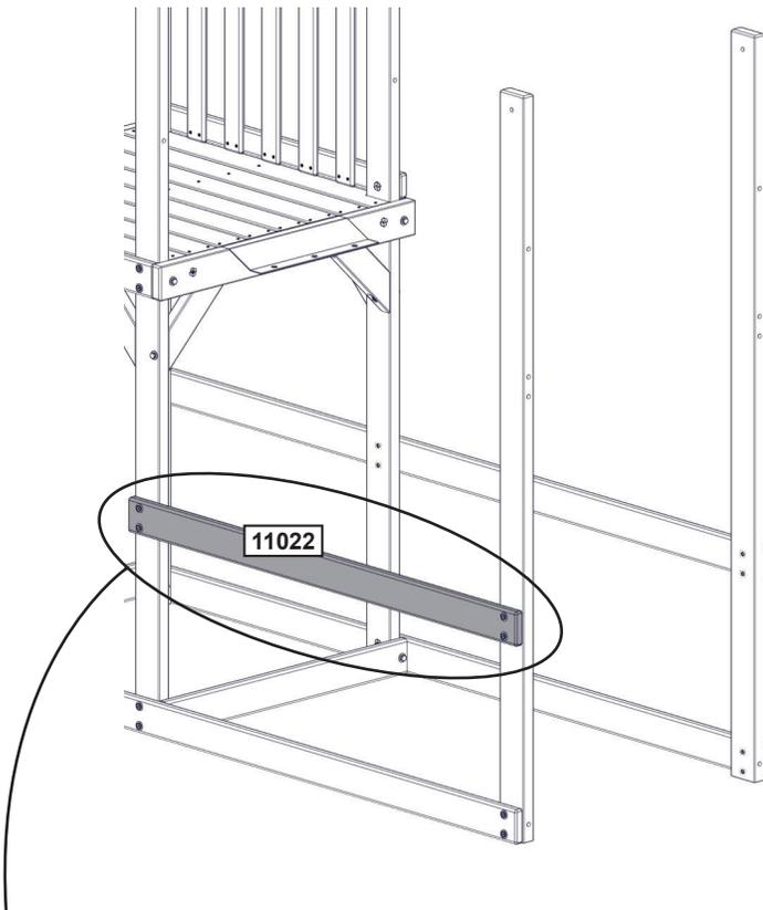
**Assemble T-Nuts first with hammer!**
