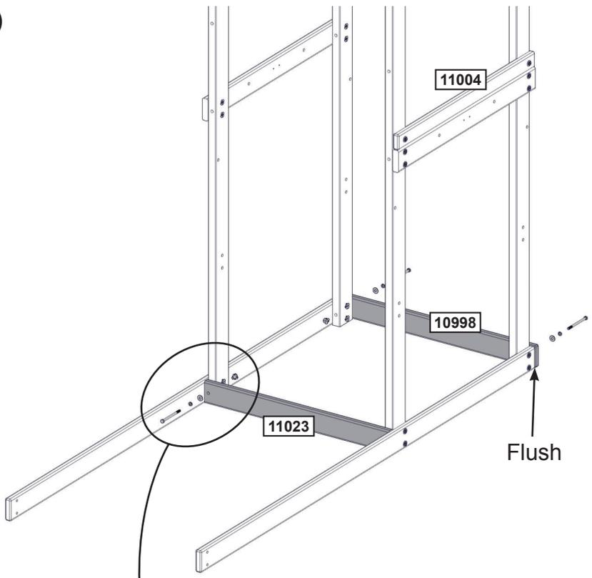
Assemble T-Nuts first with hammer!
