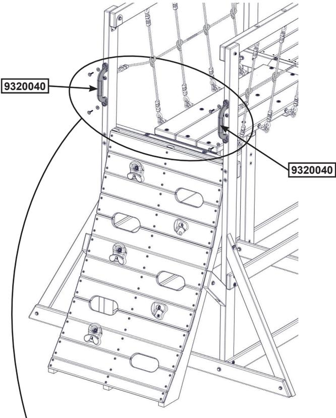
Pre-drill each hole using a 1/8" drill bit for WL3.
