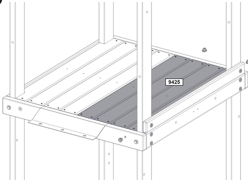
**Assemble T-Nuts first with hammer!**
