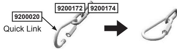
Threaded Quick Links attach to Seat and Acro Bar.
