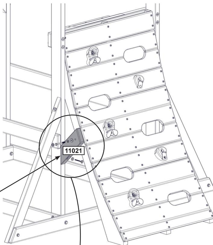
**Pre-drill each hole using a 1/8" drill bit for WL5.**
