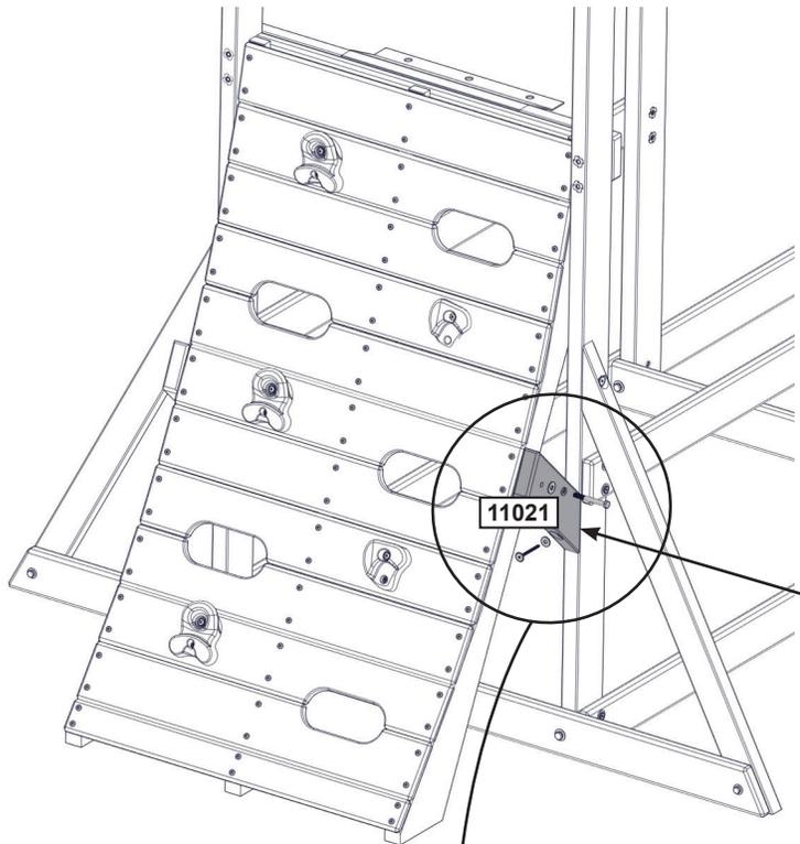
**Assemble T-Nuts first with hammer!**
