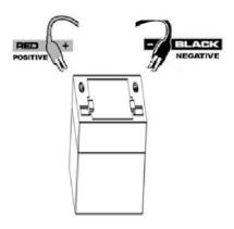
REMOVE TIMER KIT COVER AND INSTALL A 6V RECHARGEABLE BATTERY (NOT INCLUDED) BY ATTACHING RED ALLIGATOR CLIP TO THE POSITIVE TERMINAL (+) AND BLACK ALLIGATOR CLIP TO THE NEGATIVE (-) TERMINAL.
