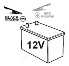
CONNECT THE DIGITAL TIMER TO A 12V RECHARGEABLE BATTERY (NOT INCLUDED) BY ATTACHING THE RED ALLIGATOR CLIP TO THE POSITIVE TERMINAL (+) AND THE BLACK ALLIGATOR CLIP TO THE NEGATIVE (-) TERMINAL.
