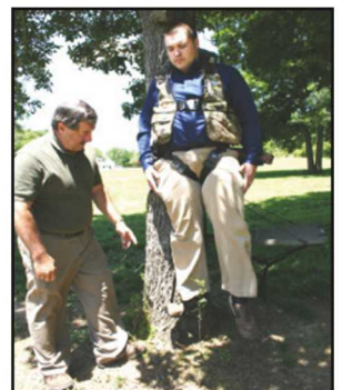
FIGURE 4: Adjust the strap to a length that will allow you to place one of your feet into it and stand relieving pressure caused by being suspended.
