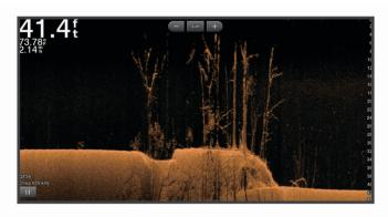
Traditional transducers emit a conical beam. The Garmin ClearVü scanning sonar technology emits two narrow beams, similar to the shape of the beam in a copying machine. These beams provide a clearer, picture-like image of what is beneath the boat.
