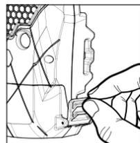
2. With the camera facing open, open the battery compartment cover by sliding the latch to the left.
