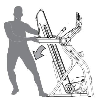
9. Grasping the Side Handrail and the front of the Upright, safely roll the treadmill to the desired location.
