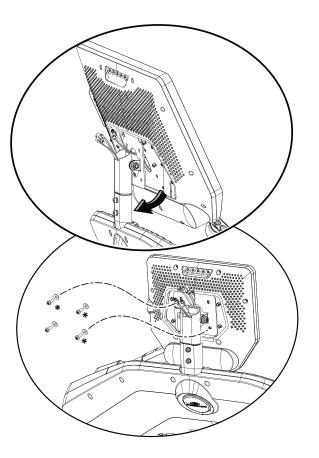
a. Place the Console onto the Console Mast and route the Cables through and out of the Console Mast
