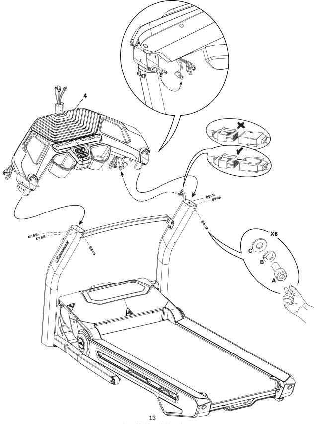
4. Attach the Upright Supports to the Frame Assembly, and Fully Tighten All Hardware
