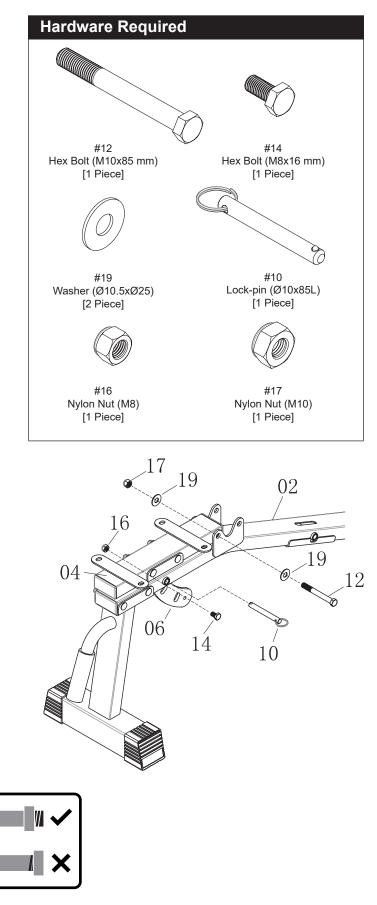
Attach Backrest Cushion Tube (#05) (now with Backrest Cushion Adjust Bracket (07)) to the Main Frame (#02), secure them together by using one Hex Bolt (#12), two Washers (#19) and one Nylon Nut (#17) from front hole on the Backrest Cushion Tube (#05) and rear hole on the Main Frame (#02) bracket.
