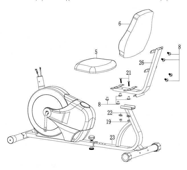
A.) Attach the Handle (#25) to Seat Support (#26). Secure it with two M8 x 1 5/8" Carriage Bolts (#21), two Ø 5/8" Curved Washers (#9), and two Acorn Nuts (#19).
