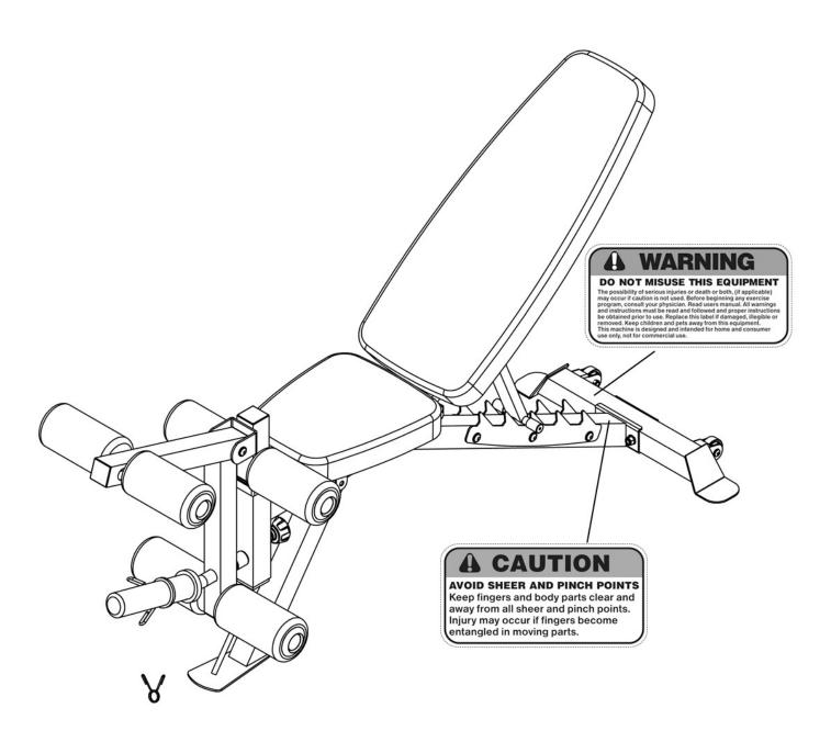
The warning labels shown here have been placed on the Rear Base. If the labels are missing or illegible, please call customer service at 1-800-999-8899 for replacements. Apply the labels in the location shown.
