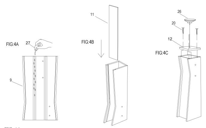
FIG: 4A Assemble the legs (#9). Run a bead of glue (#27) in the groves on the inside edges of the leg (#9).
