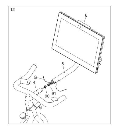
13. Tip: Avoid pinching the Wires (90, 91). Have the second person pull the console wires (F) but not the connectors out of the Console Mount (5) as you slide the Console Mount onto the Handlebar (4).
