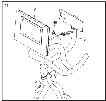
12. Connect the connectors on the Console Wire (I) to the connectors on the Mount Wire (91). Next, insert the connectors into the Console Mount (5), and then press the Wire Protector (98) into the Console Mount. **Tip: It may be helpful to insert the connectors into the Console Mount one at a time.**
