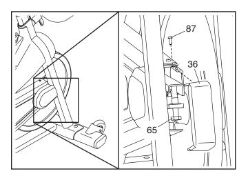
Then, tighten the M10 x 50mm Screw (65) until the Drive Belt (not shown) is tight.
