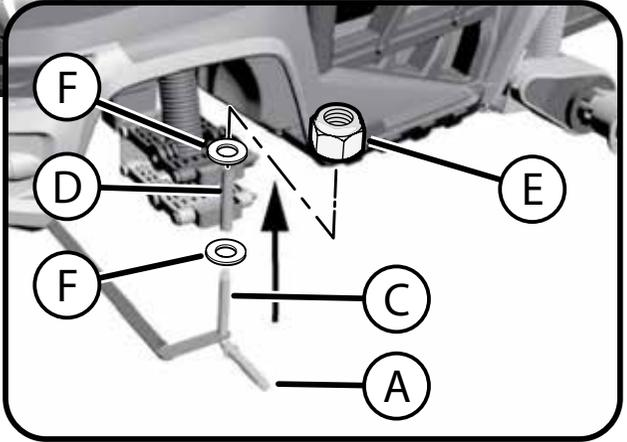
**CAUTION:** Do not over-tighten steering/axle locknuts (E)! Ensure steering/axle threads are fully into Locknut - Make sure steering is not bound up and turns easily from side to side.
