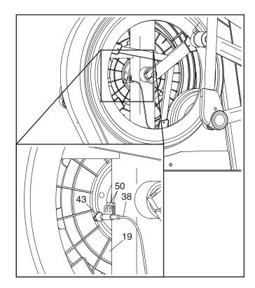
Next, slightly loosen the two indicated M4 x 13mm Self-tapping Screws (50). Slide the Reed Switch (38) slightly closer to or away from the Magnet (43), and then retighten the Screws.
