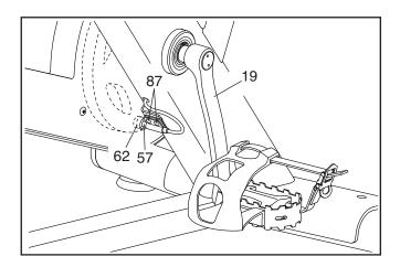
Next, turn the Left Crank Arm (19) until a Magnet (62) is aligned with the Reed Switch (57). Slide the Reed Switch slightly toward or away from the Magnet. Then, retighten the M4 x 16mm Screws (87).
