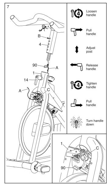
8. **See the inset drawing.** Connect the connector on the Upper Wire (90) to the connector on the Lower Wire (82).
