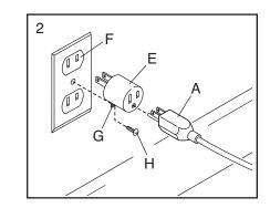
The lug (G) or wire extending from the adapter must be connected with a metal screw (H) to a permanent ground such as a properly grounded outlet box cover. **Some 2-pole receptacle outlet box covers are not** grounded. Before using an adapter, contact a qualified electrician to determine whether the outlet box cover is grounded. The temporary adapter should be used only until a properly grounded outlet can be installed by a qualified electrician.
