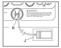
displays will light. **IMPORTANT: In an emergency**, the key can be pulled from the console, causing the walking belt to slow to a stop. Test the clip by carefully taking a few steps backward; if the key is not pulled from the console, adjust the position of the clip.
