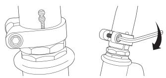
Using a 5 mm Allen wrench, check that the collar clamp bolt(s) are tightened securely. This item is tightened and quality inspected at the factory, but there is a slight chance that the effects of shipping or handling may have caused the bolt(s) to loosen.
