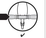
A warning: Failure to properly install and tighten the collar clamp may cause the rider to lose control and fall. If you are having difficulty understanding these instructions, please contact Razor Customer Service for assistance.
