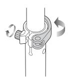
**1** To adjust the height of the handlebars, open the quick-release lever and slide the T-bar to the desired position and resecure the quick-release lever to lock into place. When the T-bar is raised to the maximum height, depress the push button located directly below the quick-release lever to unlock the T-bar.
