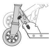
**Note:** The joint release lever is spring-loaded and will automatically lock in the upright position when fully upright.
