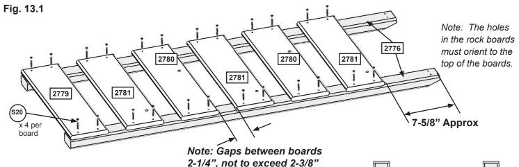
A: Lay 2 (2776) Rock Rails down, side by side with angled edges facing down. (fig. 13.1)
