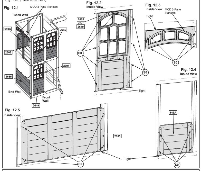
1 x 2649 Lower Window Insert 1.27 x 18.8 x 41.91" 1 x 649A Short Half Wall 1.27 x 18.8 x 20-15/16" 1 x 2665 Half Wall Insert 1.4 x 20-1/4 x 38.8"
