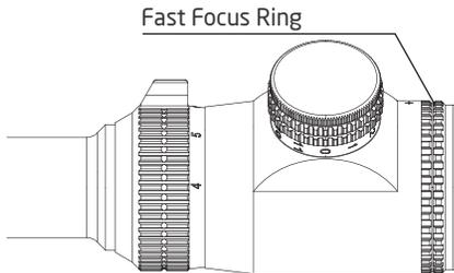
The purpose of the Fast Focus eyepiece is to focus the reticle in the scope to your eyes. For a fast focus eyepiece, just simply rotate the fast focus ring at the end of the eyepiece in either direction to get a perfect clear reticle while looking through the scope pointing at a flat plane surface. This is important to do prior to mounting.
