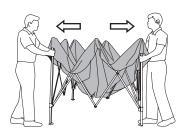
Grasp the top and bottom of the truss on opposite sides. Slightly lift canopy up and push hands together while stepping backwards until canopy is fully opened. <u>Be careful not to pinch fingers or push too hard so as to avoid damage</u> to truss.
