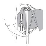
With partner, lift outer legs up and slide out the inner legs until the <u>snap button</u> locks into outer legs. Repeat on opposite legs.
