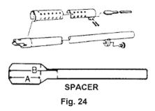
500® AND 590® MODELS 6-SHOT CUT AT 1 5/16" (A) 590® MODELS WITH ACCESSORY LUG CUT AT 1 7/8" (B) 590® MODELS WITHOUT ACCESSORY LUG, USE AS IS.
