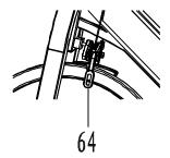
Step 8: Insert the new Left Brake Pad into the Left Holder (64).
