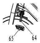
Step 4: Push Right Brake Pad (65) separated from its Holder (64) by hand.
