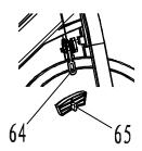
Step 6: Insert the new Right Brake Pad (65) into the Right Holder (64).
