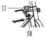
Step 10: Put down the Brake Handle (9) by Left hand; and tap the Brake Pad inside its Holder with wooden mallet (or plastic mallet) gently by right hand.
