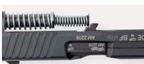
5.1.2 Fig. 6: Spring correctly seated
