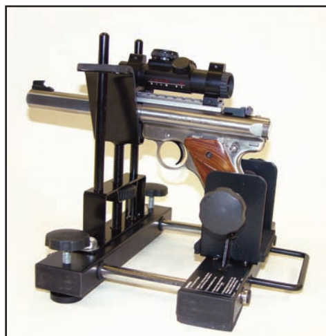
Step 5: Set the vise in the same location as when you fired. Adjust vise so that reticle is on the + Mark.
